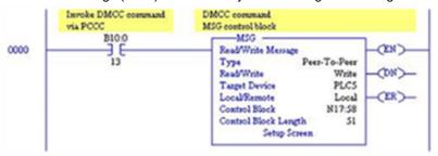
5. Enter the MSG Setup Screen and configure it as follows:
