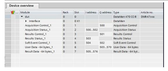
3. Remove the existing DataMan system from the hardware configuration.
